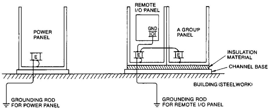
Fig. 2.14 Remote I/O Panel Insulation
