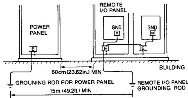
Fig. 2.12 Separation from Power Panel
