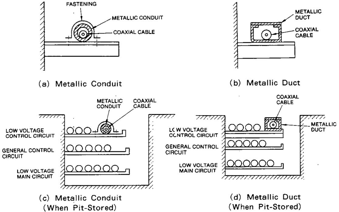
Fig. 2.6 Coaxial Cable Installation
