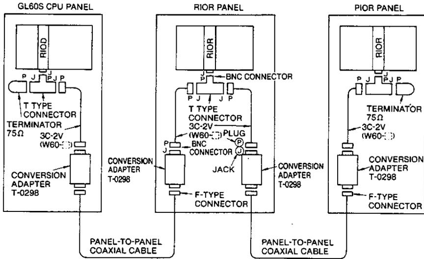
(a) CPU Panel at an End of Transmission Line
