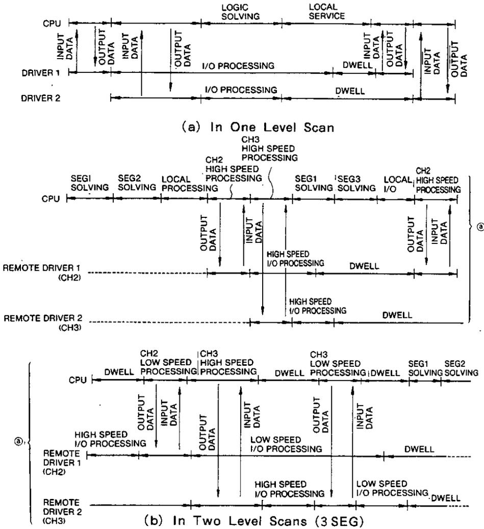
Fig. 4.5 I/O Timing of Remote I/O Channel
