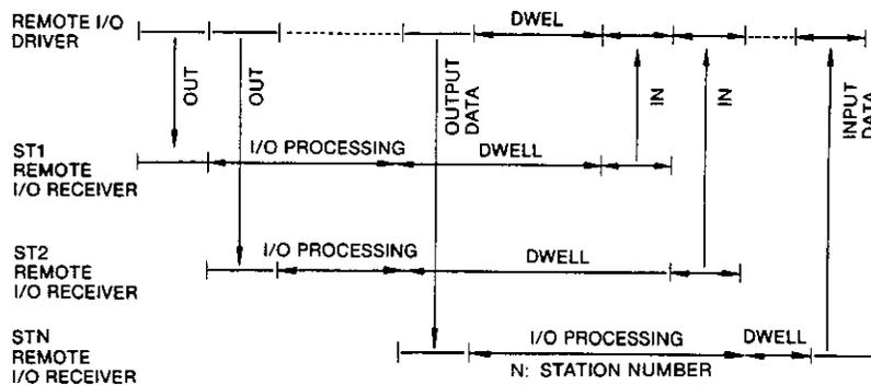
Fig. 4.6 I/O Timing of Remote I/O Station
