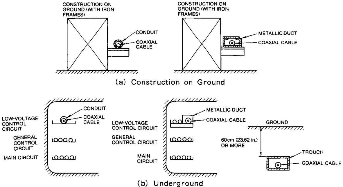
Fig. 2.9 Laying Coaxial Cables between Buildings
