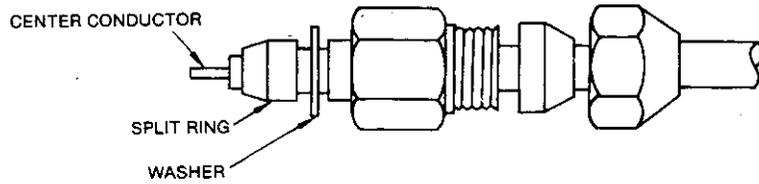
(4) Sequentially insert teflon disk and contact onto the center conductor.
