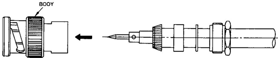
Note: Insert the contact into the body to the end.
