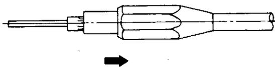
(3) Press a ferule into the coaxial cable.
