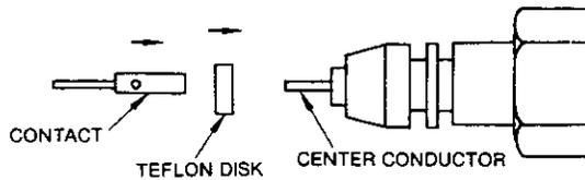
(5) Press to bond the contact, using a 9.5 mm coaxial-cable press-pliers.
