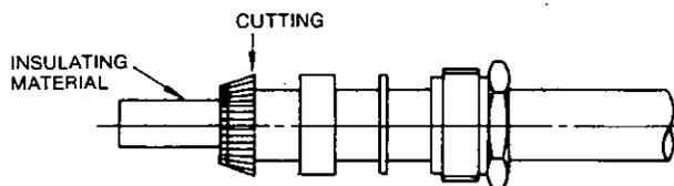
(4) Remove the insulating material, leaving about 3mm, to expose the core. Cut the core leading end, so that the bare core is 3mm.
