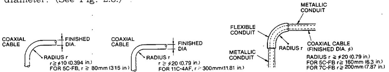
Fig. 2.7 Cable Bending
