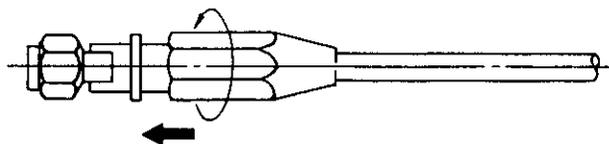
Note: Fix the body and turn the nut for tightening.
