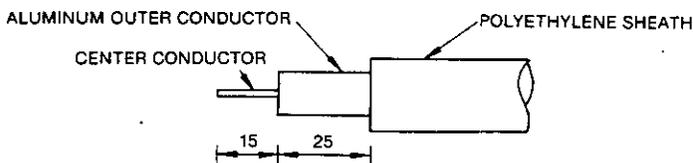
Note: Be careful not to bend or damage the center conductor.
