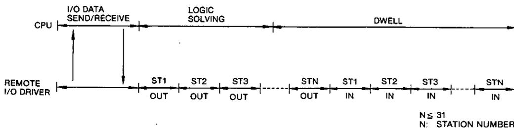
Fig. 4.1 Logic Solving and I/O Processing
