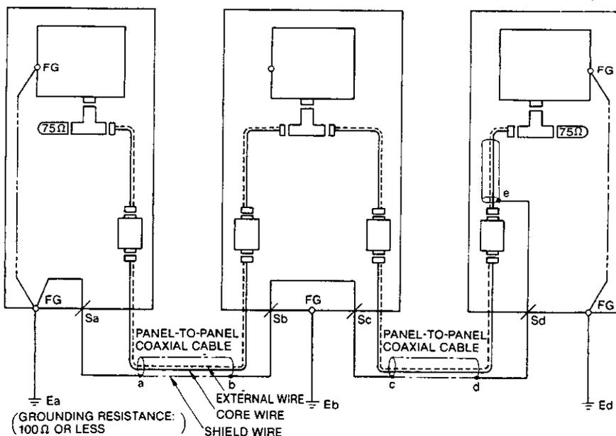
Fig. 2.11 Example of Coaxial Cable Grounding
